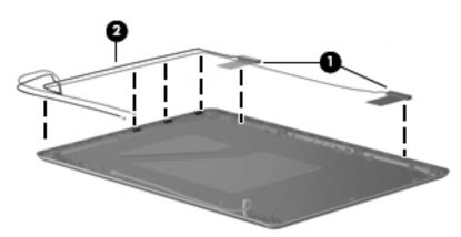
Reverse this procedure to install the WLAN transceivers and cable.
